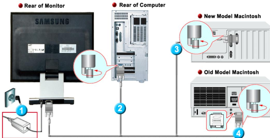
1. Connect the DC Adapter for your monitor to the power port on the back of the monitor. Plug the power cord for the monitor into a nearby outlet.
