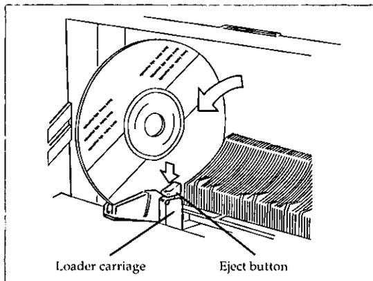
**Setting/Removing discs****How to set discs****A**
