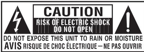
**WARNING : TO REDUCE THE RISK OF ELECTRIC SHOCK, DO NOT REMOVE COVER (OR BACK). NO USER SERVICEABLE PARTS INSIDE. REFER SERVICING TO QUALIFIED SERVICE PERSONNEL.**
