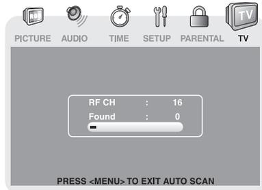
3. Use the **<=>** button to select Auto Scan, then press the **>** button to enter auto scan menu. Use the **<=>** button to select Start to Scan, press the **>** button to begin scanning. (If you selected CATV on Step 2, you need to select Cable System before Start to Scan). The system will automatically start to scan and preset all available TV channels.
