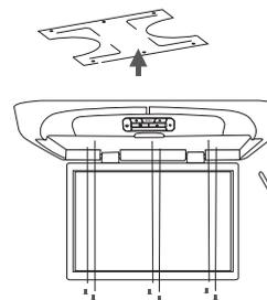
4. Flip the monitor screen down and tighten the monitor to the support bracket, using the supplied screws.
