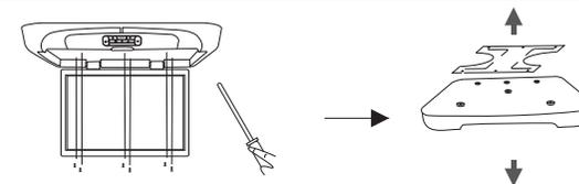
2. Tighten the metal support bracket to the ceiling support beam(s), using the supplied screws. Take extra care to not penetrate the roof of your car.
