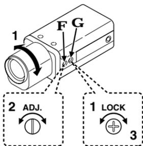
**F** Flange-back adjustment screw (**FLANGE BACK ADJ.**)
