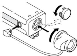
A 1/3 inch CS mount type lens without EE amplifier circuit that only uses a DC power source. This camera can receive (the **A.I. LENS** switch to the DC type) a CS mount type lens without the need of an adaptor.
