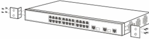
**Figure 2-1** Fix the mounting ears
