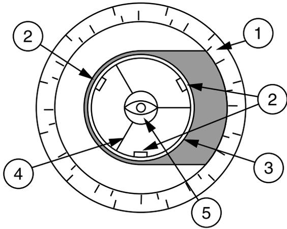
**Fig. 7:** Correct Collimation.
