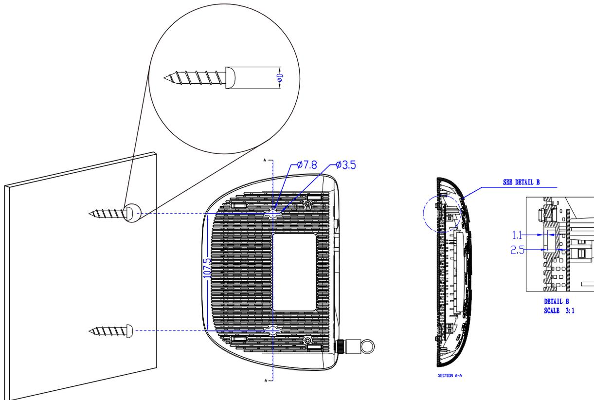
Figure 2-3 Wall-mount Install
