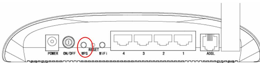
**Step 2:** Press and hold the WPS button of the adapter directly for 2 or 3 seconds.
