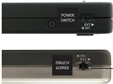
Switch between internal power through USB connection or external power using included USB power cable or 110/220 5V power adapter
