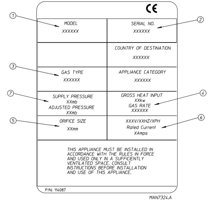
When contacting Maytag, the information on the data label is required to ensure proper service/parts assistance. The data label is located at the upper left rear of the dryer behind the back guard.
