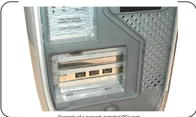
*Example of a properly installed PCI card.*
