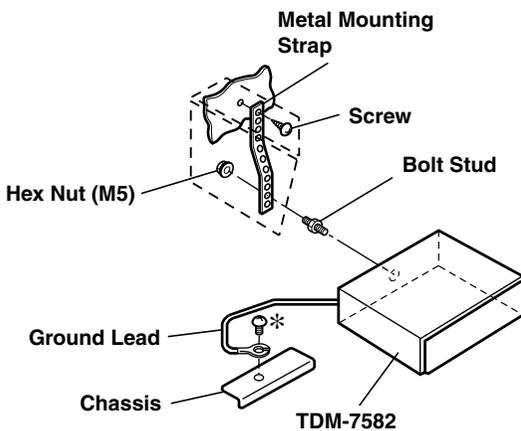
Reinforce the head unit with the metal mounting strap (not supplied). Secure the ground lead of the unit to a clean metal spot using a screw (\*) already attached to the vehicle's chassis. Connect each input lead coming from an amplifier or equalizer to the corresponding output lead coming from the left rear of the TDM-7582. Connect all other leads of the TDM-7582 according to details described in the CONNECTIONS section.
