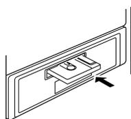
When the cassette is loaded, the player automatically starts tape playback and indicates "TAPE" in the display.
