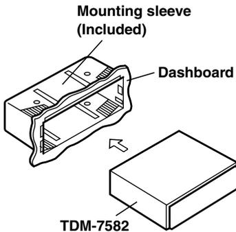
Remove the Detachable Front Panel (refer to page 4). Slide mounting sleeve from main unit. Slide the mounting sleeve into the dashboard.
