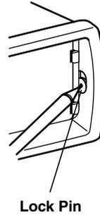
Slide the TDM-7582 into the dashboard. When the unit is in place, make sure the locking pins are fully seated in the down position. This can be done by pressing firmly in on the unit while pushing the locking pin down with a small screwdriver. This ensures that the unit is properly locked and will not accidentally come out from the dashboard. Install the Detachable Front Panel.
