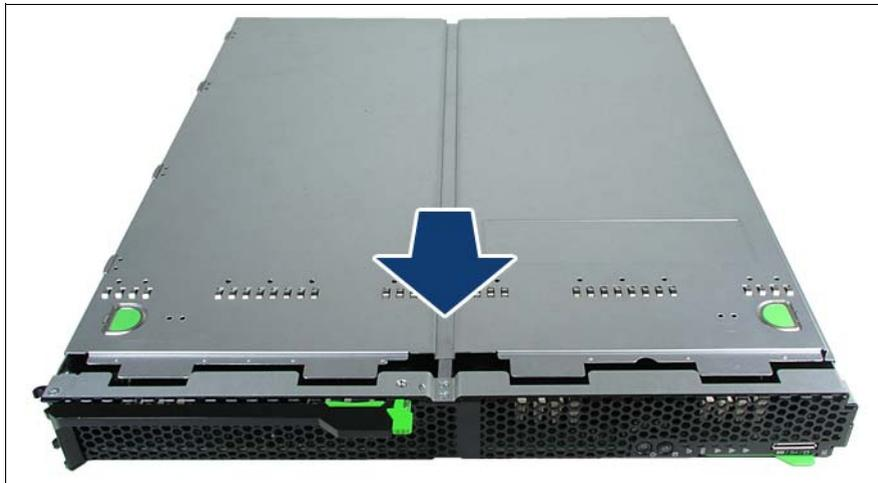
Figure 16: Closing the server blade
