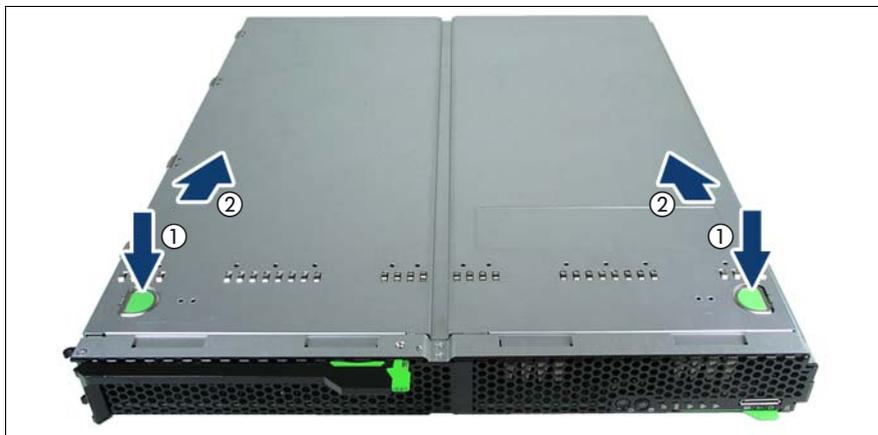
Figure 9: Removing the cover
