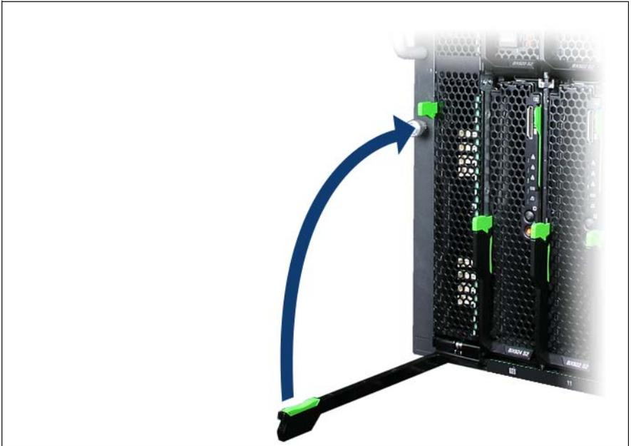
Figure 4: Locking the Server Blade
