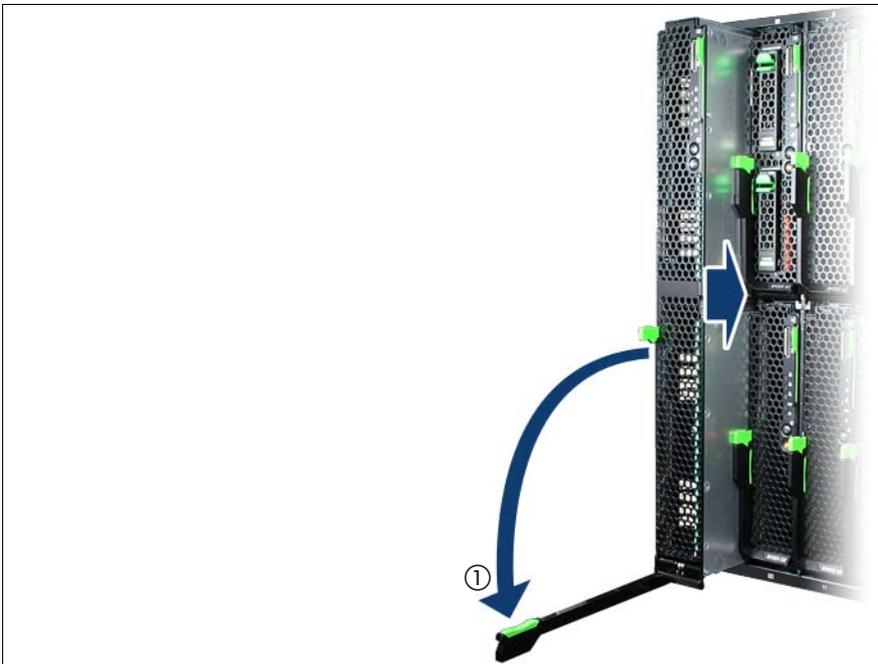
Figure 3: Installing the Server Blade
