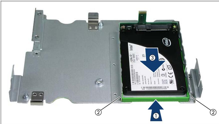
Figure 11: Removing the SSD drive mounting frame.
