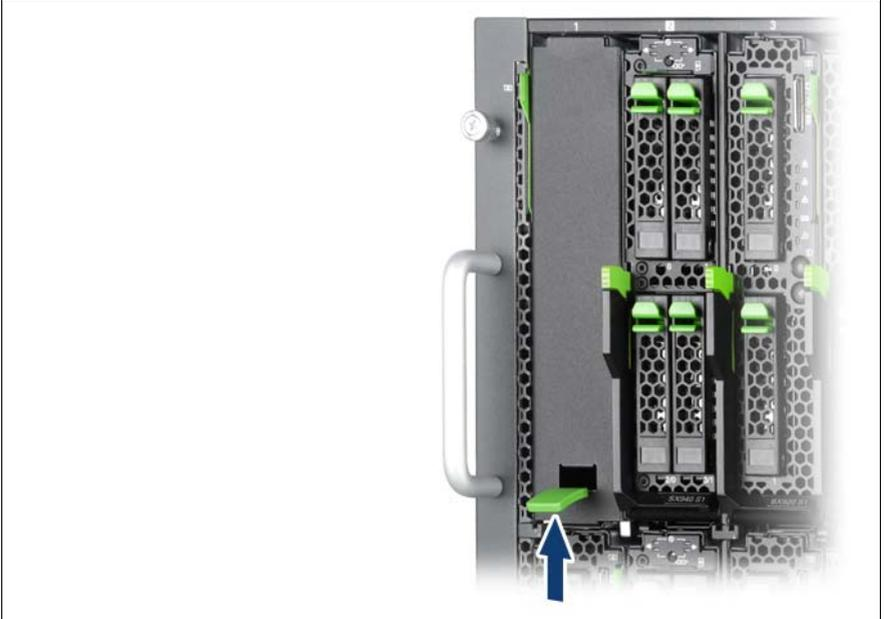
Figure 2: Removing the server blade dummy module
