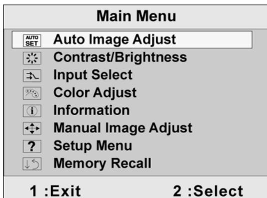
**NOTE:** All OSD menus and adjustment screens disappear automatically after about 30 seconds. This is adjustable through the OSD timeout setting in the setup menu.
