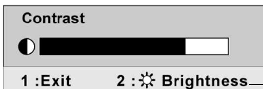
The line at the bottom of the screen shows the current functions of buttons 1 and 2: Exit or select the Brightness control.
