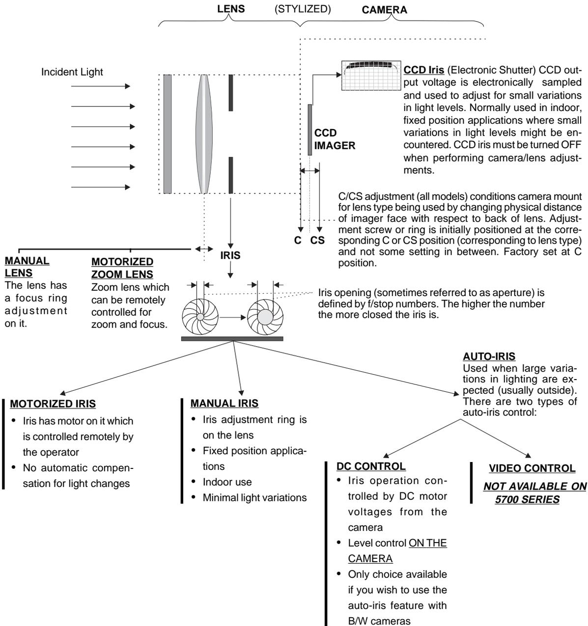
The purpose of backfocusing is to make the adjustments necessary for the picture to remain in focus throughout the camera's zoom range, which is the case for instance, in motorized zoom, auto iris configurations. Manual Iris lens/camera combinations also need to be backfocused. Follow the general instructions listed below to adjust backfocus appropriate to your camera/lens combination.
