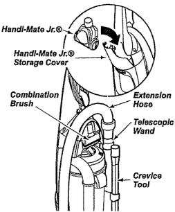
Remove crevice tool from the wand by twisting. Place in wand holder.
