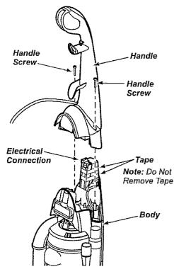
tion below When installing the handle, firmly press the handle onto the body. Secure with handle
