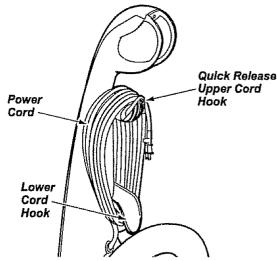
Wrap the power cord around the upper and lower cord hooks and lock the power cord plug onto the power cord.
