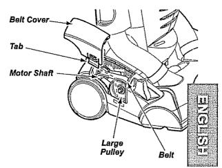
Reinstall belt cover and securely snap into place.
