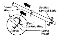
Extend the wand to its full length. Turn the locking ring counter-clockwise to the **LOCK** position. Attach the extension wand onto the open end of the hose.
