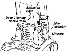
Visually inspect the hose and the base area into which the hose is connected.
