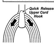
Turn the quick release upper cord hook to either side and down to release the power cord.
