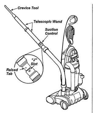
To achieve maximum reach with the attachments, add the crevice tool to the end of the wand by inserting and twisting slightly.
