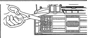
To clean agitator turn vacuum over, cut off any carpet pile and lint entangled around agitator with a pair of scissors in the slots provided. Remove hair, string, lint and other debris from the agitator.
