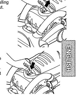
Replace lens cover by inserting bottom tab of lens into slot then applying pressure to top tabs with a screwdriver. A "popping" sound indicates lens is snapped properly in place.
