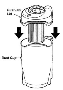
Replace dust bin lid assembly by placing back on dust cup as shown.
