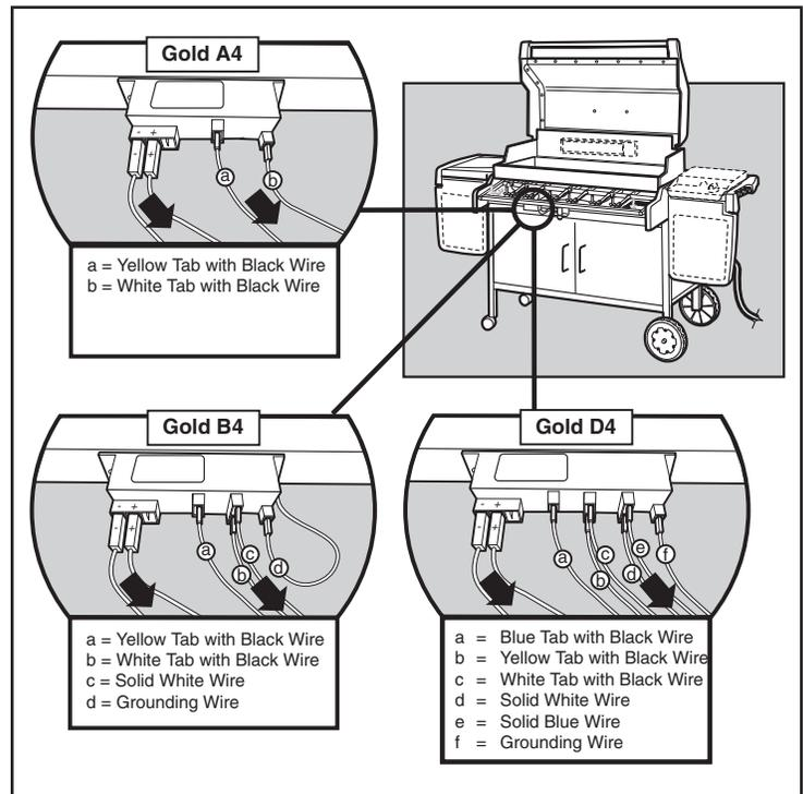
8. Disconnect all ignition wires from the Ignition Module.
