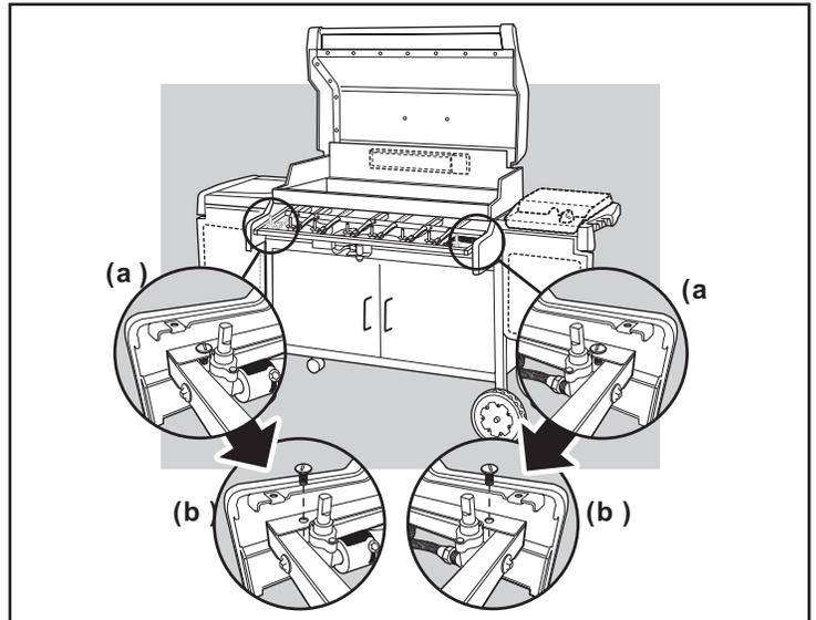
11. Pull manifold assembly out from the manifold frame.
