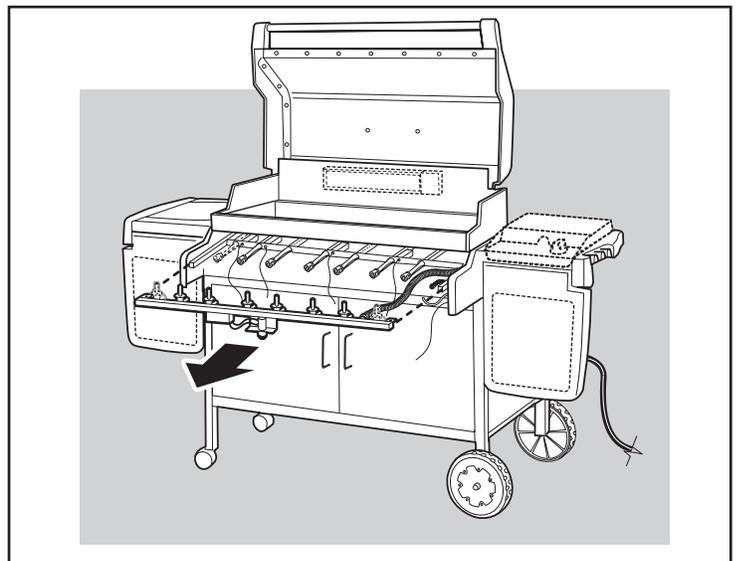
12. Lift and twist the burner assembly slightly, to separate the Crossover® tube (a) from the burners (b).
