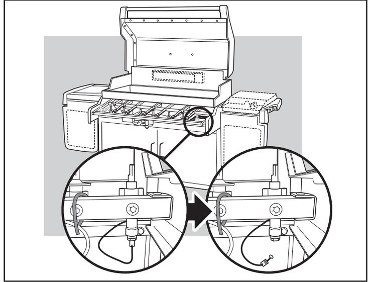
9. Disconnect the Thermocouple from the IR Burner valve.
