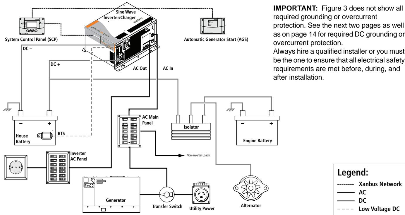
**IMPORTANT:** Figure 3 does not show all required grounding or overcurrent protection. See the next two pages as well as on page 14 for required DC grounding or overcurrent protection.
