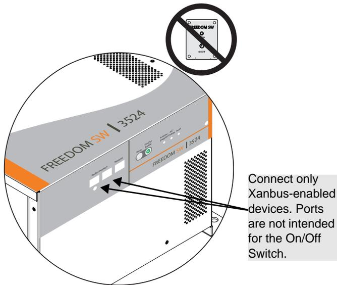
**Figure 14** Connecting to a Xanbus Network Port
