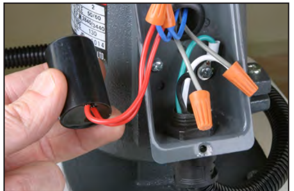
Figure 50. Pump motor wiring and capacitor (M2).
