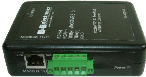
Figure 4. MES1B Serial Connector
