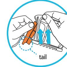
Hold the Head portion (1 in the drawing) of the silicone blade and slide downward to the middle of the blade slot, then pull outward.
