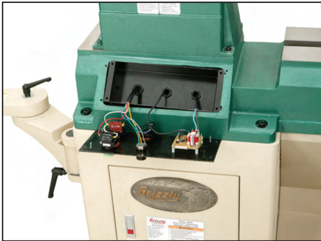
Figure 72. Control panel wiring.
