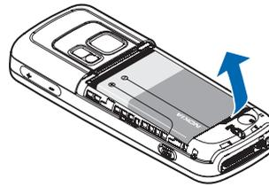
After you have removed the back cover, insert your finger into the finger grip, and lift the battery from its compartment.
