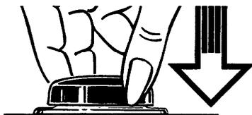
The burner ignites automatically. Turn the knob either direction to adjust the flame size.
