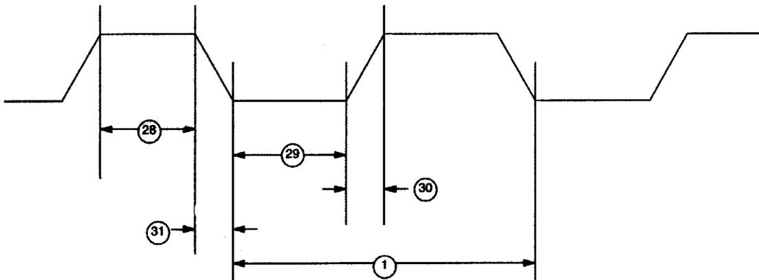
**AC CHARACTERISTICS (continued)****POWER CYCLE TIME** $(T_A = 0^\circ\text{C to } +70^\circ\text{C}; V_{CC} = 5V \pm 10\%)$
