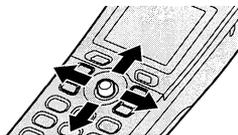
It can also be used to select the center soft key icon (page 18), by pressing down on the center of the joystick.
