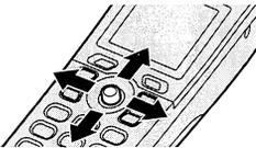
It can also be used to select the center soft key icon, by pressing down on the center of the joystick.
