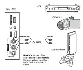
3 Connect the audio connectors of the AV cable (the red and white connectors) to the AV OUT AUDIO jacks of the external device, then connect them to the AV IN AUDIO-L and AUDIO-R jacks on the side of your TV.
