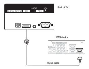
**Note:** To connect a DVI device, use a DVI to HDMI adapter cable to connect to the **HDMI** jack on the TV, then connect an audio cable to the **PC IN AUDIO** jack on the back of the TV.
