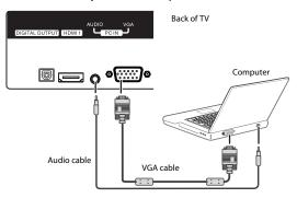
3 Connect one end of an audio cable (not included) to the PC IN AUDIO jack on the back of the TV, then connect the other end of the cable to the AUDIO OUT jack on the computer.
