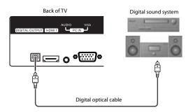
3 Connect the other end of the audio cable to the digital optical input jack on the digital audio system.
