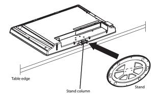
3 Align the locators on the stand column with the locating holes on the stand, then secure the stand to the column with the four M5 screws (provided).
