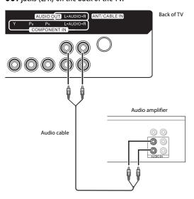
**Note:** Cable connectors and jacks are often color-coded. Match the colors when you connect the AV cable.
