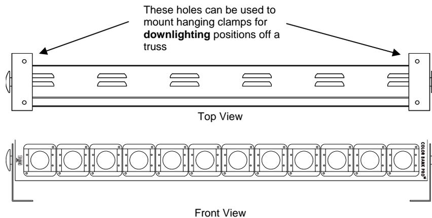
The CH-175 can also be used for **uplighting**. The yoke hardware can equally serve as floor stands.
