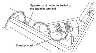
2 Thread the speaker cord through the gap along the side of the subwoofer.
