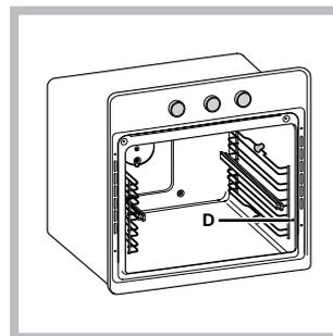
3. Secure the two frames with the guide rails using the holes provided on the oven walls (see diagram). The holes for the left frame are situated at the top, while the holes for the right frame are at the bottom.
