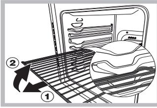
**WARNING!** The oven is provided with a stop system to extract the racks and prevent them from coming out of the oven (1).
