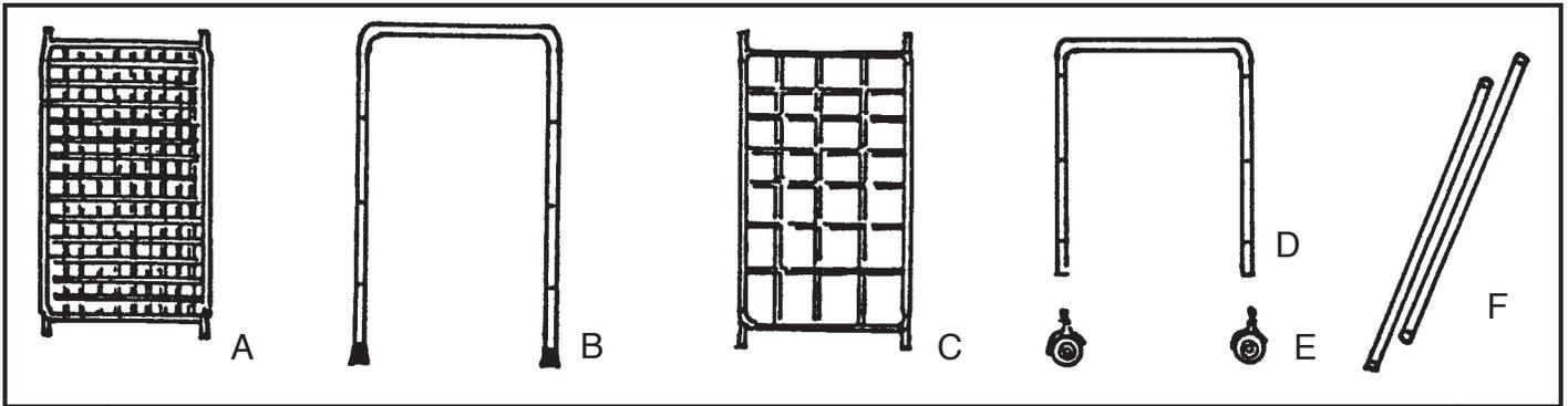
1. Attach grid tray with small openings(A), to bottom of large frame section(B).
