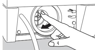
6. Replace cover (insert stud on the cover into the guide slot) and tighten in a clockwise direction.
