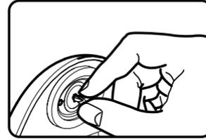
UNSCREW THE BAG PUNCTURE COUNTERCLOCKWISE TO RELEASE IT. THE BAG PUNCTURE IS SHARP. USE CARE WHEN HANDLING IT.
