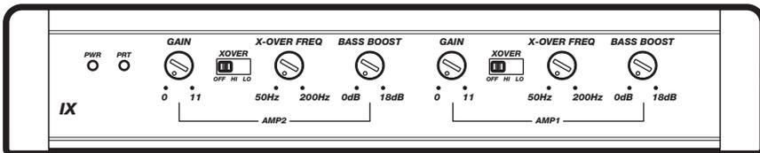
**Input Gain Control:** The input gain control is not a volume control. It matches the output of the source unit to the input level of the amplifier. Turn the source unit up to about 3/4 volume (if the source unit goes to 30, turn it to 25). Next, slowly turn (clockwise) the gain on the amplifier up until you can hear audible distortion, then turn it down a little.
