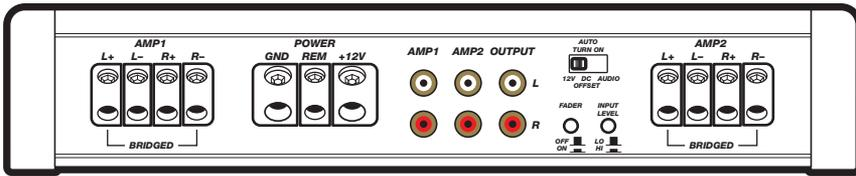
**Automatic Turn-On Selection:** The IX series offers three different automatic turn-on modes that can be selected on the end panel; +12V, DC Offset, and Audio. Using either the DC Offset or Audio mode causes the REM terminal to have +12V out for turning on additional amplifiers.
