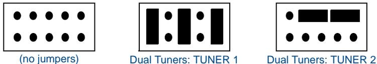
FIG. 61 Tuner Module Jumper Configuration (Red Interface Boards)
