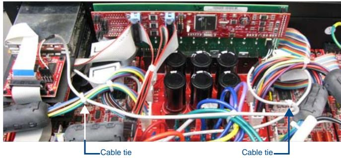
**FIG. 71** Cable Routing
