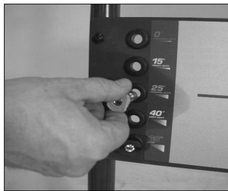
Figure 3 - Insert spray tips into the holder
