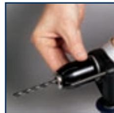
**WARNING.** Do not attempt to tighten the chuck by gripping the front part and turning the drill on. Damage to the tool and personal injury may result. Be sure to tighten the chuck with the spindle lock button held pressed to achieve maximum tightness.
