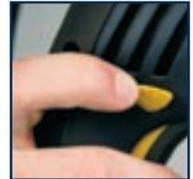
**CAUTION.** Any attempt to reverse the direction of rotation whilst the drill is turning is likely to permanently damage the motor, gearing or both.
