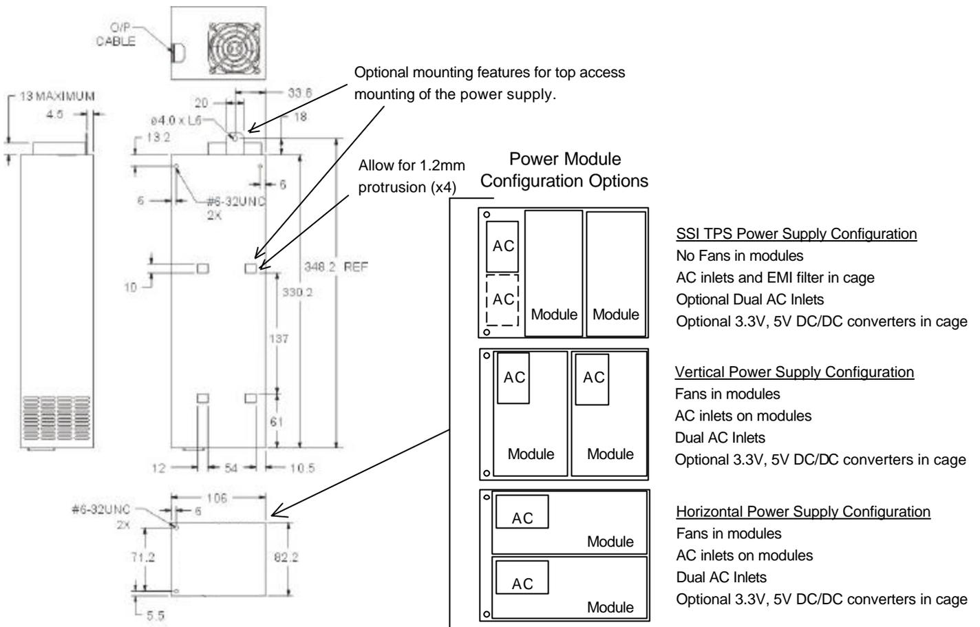
Figure 1: Enclosure Drawing
