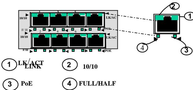
per the IEEE802.3af PoE standard. The Power Pass-through PoE modules are totally dependent upon the powerful -48VDC input power supply to support more RJ-45 (10/100) ports. Each port requires atleast 15watts to power up the PoE PD devices. Maxm. one PoE modules can be configured in the A, B slot of any 6K16 s with -48vdc power input. The PoE modules are also
