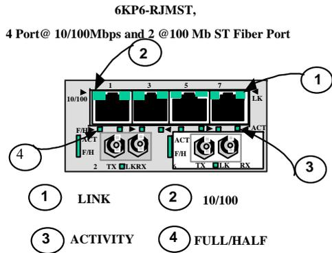
Each port has an Activity (ACT) LED indicating packets being received, a Link (LK) LED that indicates proper connectivity with the remote device when lit, and FDX/HDX LED to indicate full-duplex mode when lit (or half-duplex when off). The 10/100 LED indicates the speed, if the LED is ON 100Mbps if it is OFF 10Mbps.
