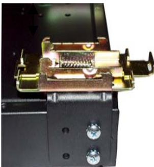
The Din Rail Latching clips are mounted on the upper rear corners of the 6K16V unit. Two threaded holes are provided on the sides of 6K16V for DIN-Rail mounting purposes. See side view at the left, with the top of the unit pointed to the right. The required two screws are included with the DIN-Rail brackets, and are no.10-32 X 3/8 PHIL. PAN w/star washer. The two heavy duty Din-Rail latches are designed as if that they can be manually accessed from
