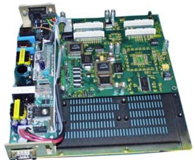
**Figure 3.6.1b: Magnum 6K16-Series, Top view without chassis cover**
