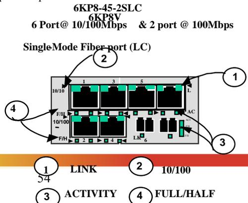
When installed in a Magnum 6K16-Series Switch, it supports the standard distances as mentioned on 5.2.4. and the LEDs also act similarly.
