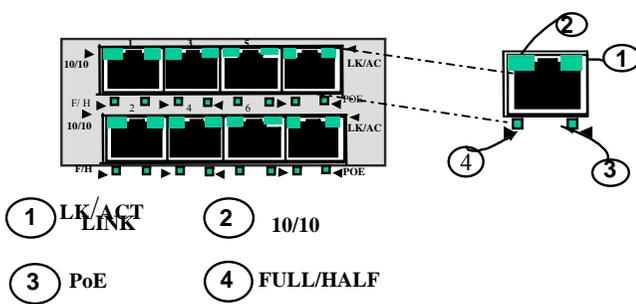
IEEE802.3af PoE standard. The Power Pass-through PoE modules are totally dependent upon the powerful -48VDC input power supply to support more RJ-45 (10/100) ports. Each port require atleast 15watts to power up the PoE PD devices. In this Fig. the top 8-RJ45 ports are enhanced with POE option The 8-RJ45
