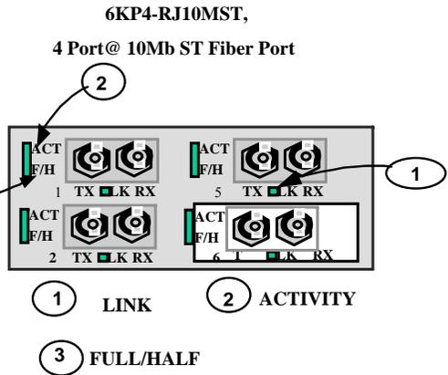
hub to connect to the switch through 10Mb fiber ports. It supports distances according to the 10Base-FL standard i.e, 2Km distance for multi-mode fiber. (Single-mode for 10Km distance may be available as a special order).
