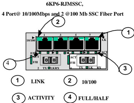
module of the 6K16-Series Switch supporting four Copper and two single-mode fiber network segments.
