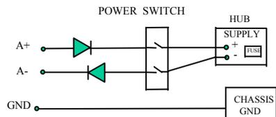
incorrect polarity connection, for example, will neither affect the Switch, its internal power supply, nor will it blow the fuse in the internal power supply.
