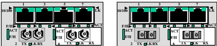
SC or single mode SC or Long Reach SC ports. For ports numbering, ports 1,3,5,7 are copper, ports 2 and 6 are fiber, ports 4 and 8 are not present.
