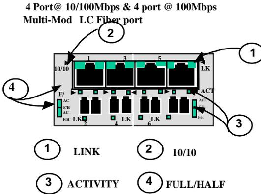
The Magnum 6KP8-45LC Module is a combo module with a combination of copper and Fiber (Small Form Factor) LC type ports. The small size of LC connectors allows an advantage of having more
