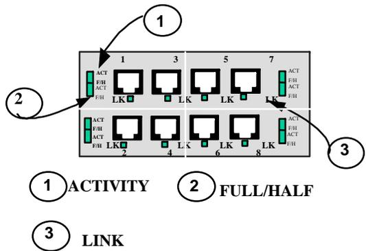
The functionality of this 100BASE-FX multi-mode 8 Port module is essentially the same as the ST and SC-types. It has the same LEDs per port indicating port activity (ACT), Link (LK), and FDX or HDX operation.
