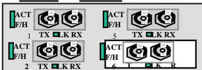
The 4-port @10Mb ST fiber modules behave the same as the 4@100Mb ST fiber modules except for the 10Mb speed. For ports numbering, ports 1, 2, 5, 6 are present, ports 3, 4, 7, 8 are not present. There is also a similar 100Mb fiber SC module.
