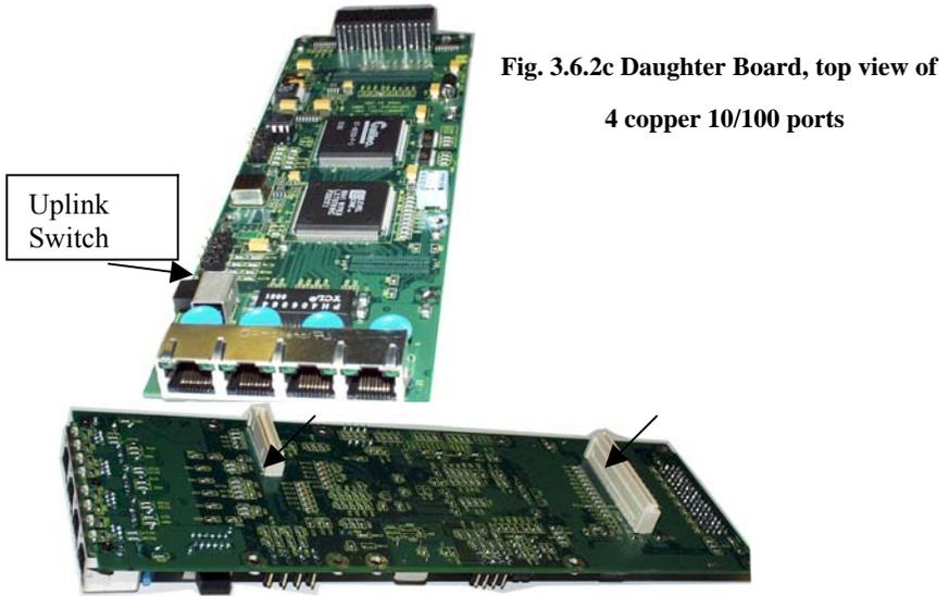
**Fig. 3.6.2c Daughter Board, top view of 4 copper 10/100 ports**
