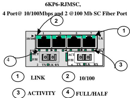
While the functionality of these two modules is essentially the same, the 6KP6-RJMSC is equipped with an SC-type "snap-in" connector instead of an ST-type.
