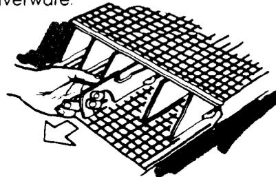
**To remove the basket**, slide it toward the top of the door – by the handle. Lift it off the holding buttons. Replace it in reverse order.
