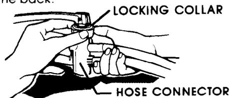
3. Pull down on the locking collar while lifting the hose connector onto the faucet adapter.
