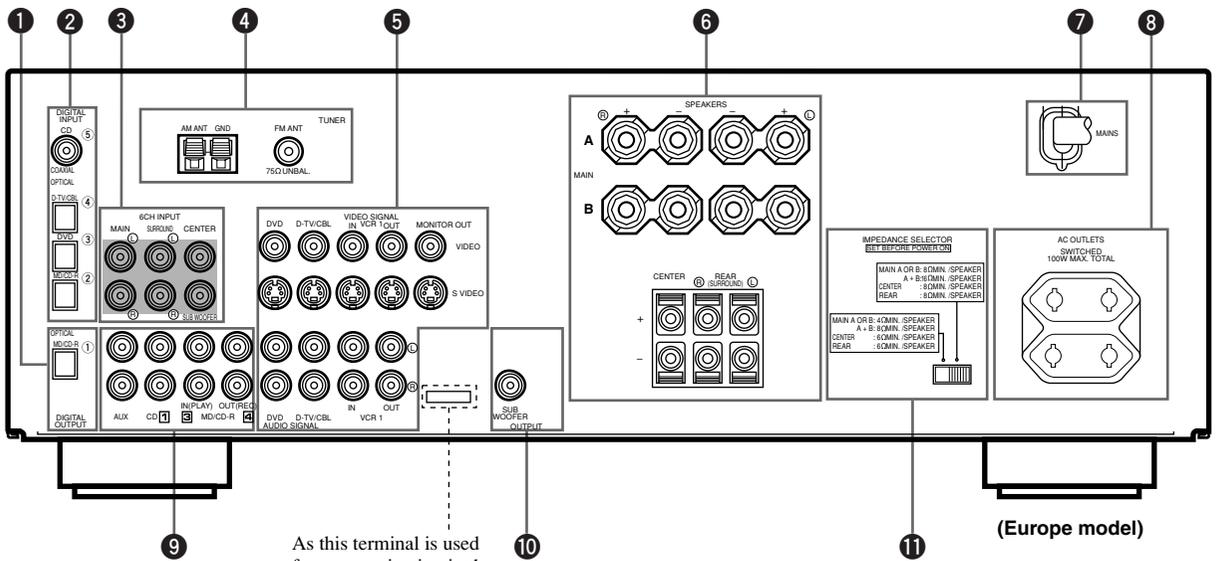
As this terminal is used for an examination in the factory, do not connect any equipment to this terminal.
