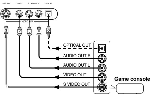
These jacks are used to connect any video input source such as a game console to this unit.
