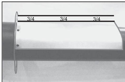
**Figure 5.34** When installing the trim ring/heat shield assembly make sure the trim ring is centered in the hole and that the shield is above the pipe. There must be a minimum of 3/4 in. (19mm) minimum clearance maintained to combustibles from the top of the heat shield.
