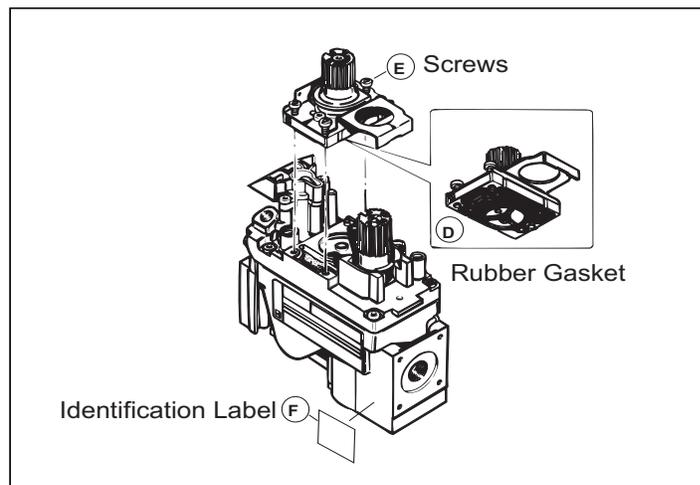
**Figure 6.6** Ensure that the rubber gasket (D) is properly positioned and install the new HI/LO pressure regulator assembly to the valve using the new screws (E) supplied with the kit. Tighten screws securely. (Reference torque = 25 in./lb.) Install the enclosed identification label (F) to the valve body where it can be seen.
