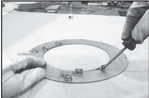
**Figure 5.31** Lay the trim ring on flat surface and bend up the six welded brackets into a 90 degree position. The brackets along the outer edge of the ring are for locating the ring in the center of the hole.
