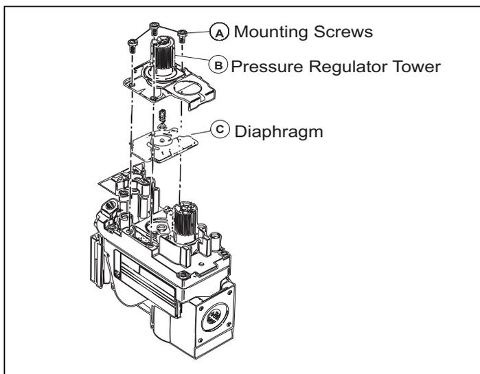
**Figure 6.5** Turn control knob to the OFF position, ensure that gas supply to the valve has been turned off. Using a Torx TH20, or slotted screwdriver, remove the three pressure regulator mounting screws (A), pressure regulator tower (B), and diaphragm (C).
