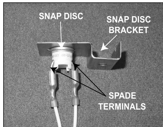
**Figure 8.15** Install the snap disc. A snap disc bracket is located in the appliance's component bag. Bend the two spade terminals on the snap disc from a horizontal to a vertical position. Insert the snap disc through the hole in the snap disc bracket and attach the two white wires from the wiring harness to the snap disc.
