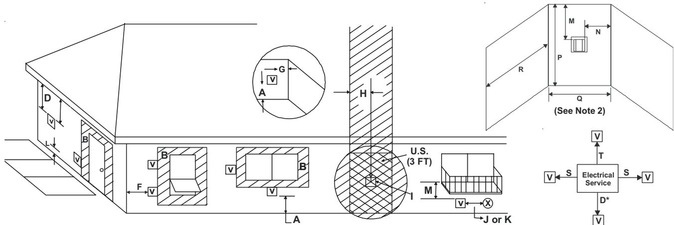
**V** = VENT TERMINAL      **X** = AIR SUPPLY INLET      **▨** = AREA WHERE TERMINAL IS NOT PERMITTED
