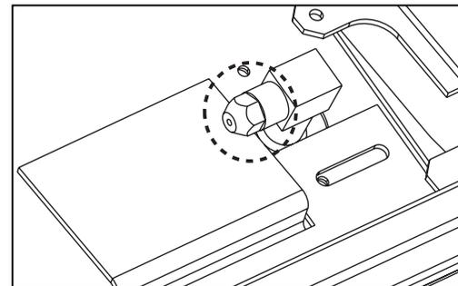
**Figure 6.4** Remove main burner orifice using a 3/8 in. wrench. Be sure to align notch on left side of pilot hood, shown. Replace orifice with the proper size as indicated below for your gas type and venting.
