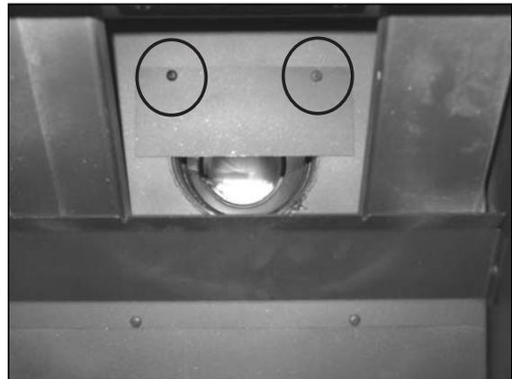
**Figure 8.5** With the baffle removed, remove the two screws located in the back of the firebox. Reuse the screws to install the flue restrictor. Reinstall the baffle using the two screws previously removed.
