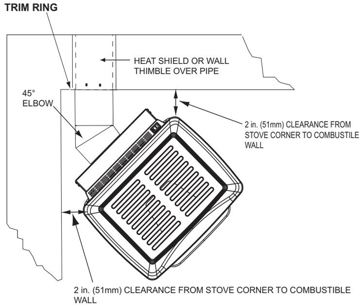
**FIG. C MINIMUM CLEARANCE**
