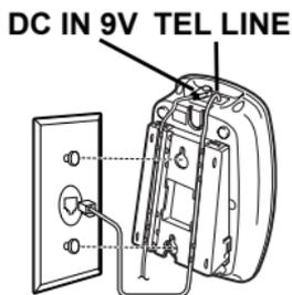
4. Route the adapter and modular cords through the bracket's grooves.
