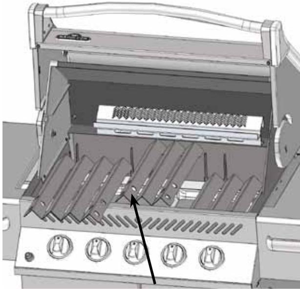
*Ensure holes in sear plates are positioned to the front of the grill.*
