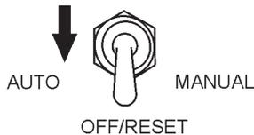
**Figure 54. MPEC Control Switch (Off/Reset)**
