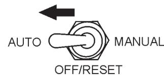
**Figure 52. MPEC Control Switch (AUTO)**
