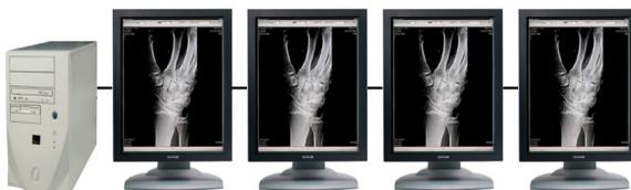
An example of a medical viewing station consisting of one PC with four imaging board heads and four Barco flat panels connected. Those panels have an internal optical sensor.
