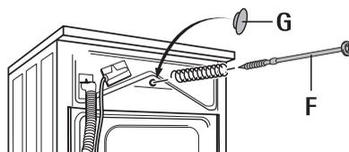
**Important!** Press in the cap with sufficient strength so that it engages in the rear panel (protects the inside of the unit against splash water).
