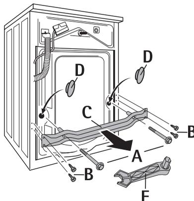
**Important!** Press in the caps with sufficient strength so that they engage in the rear panel (protects the inside of the units against splash water).
