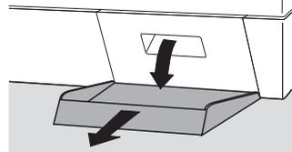
**3.** Remove the emergency drainage hose from its holder.
