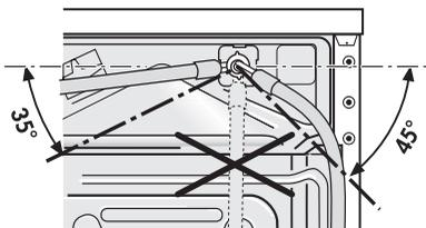
**2.** Connect the hose with the straight connection to a water valve with a screw thread R 3/4 (inches).
