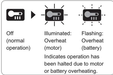
To protect the motor or battery, be sure to note the following when carrying out this operation.
