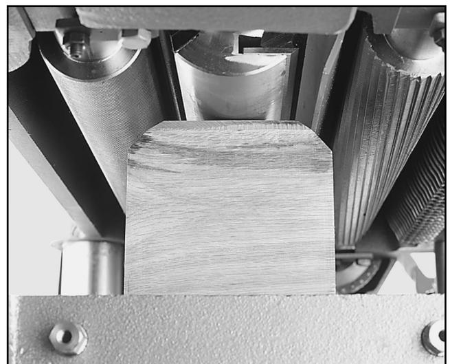
**Figure 11.** Guide block indicates parallelism.
