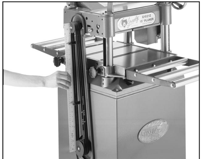
**Figure 31.** Checking pulley alignment.
