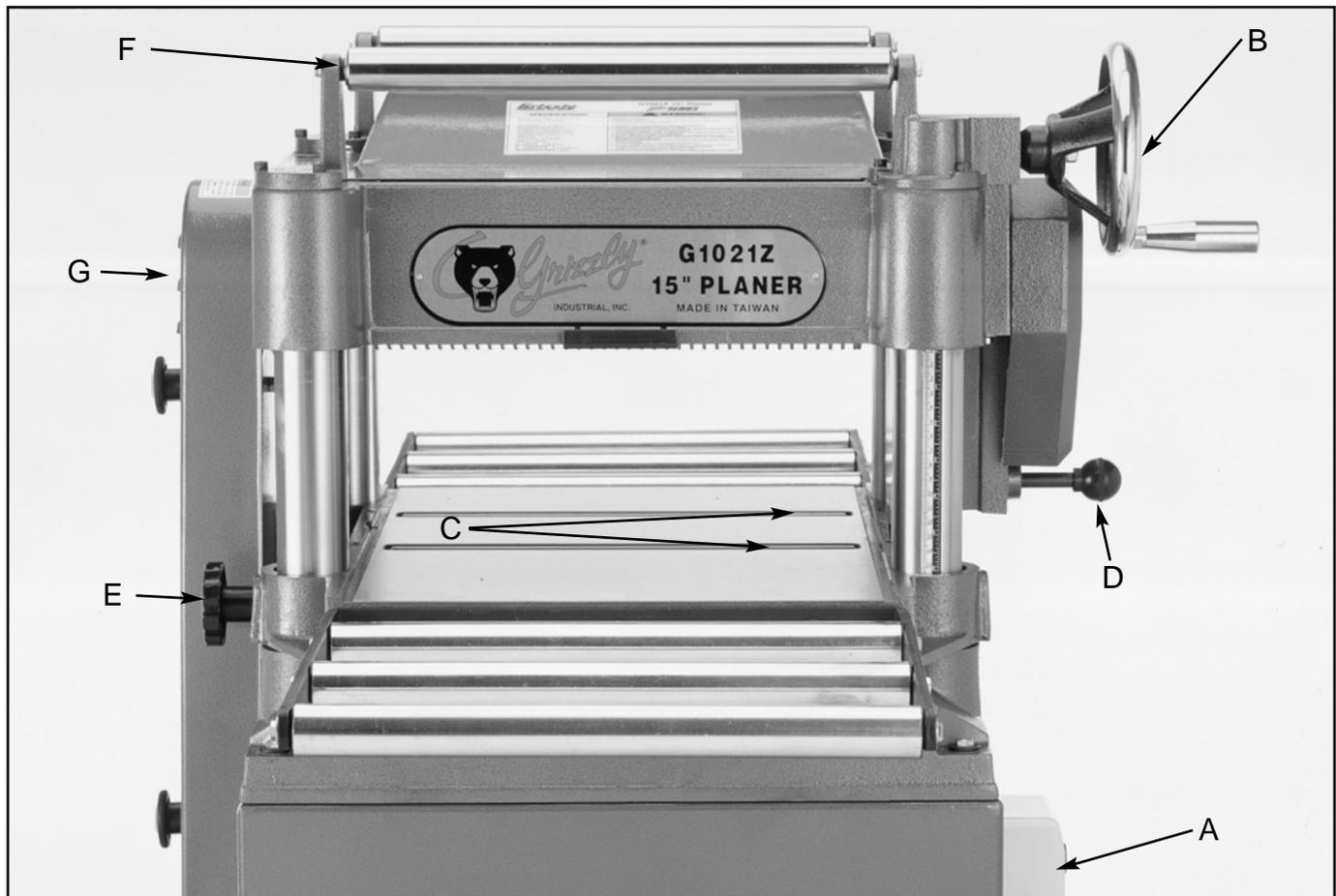
**Figure 9.** Overview of planer adjustment controls.
