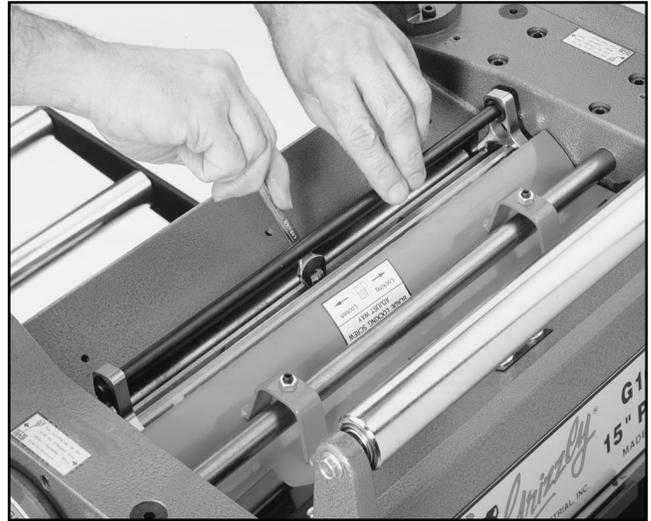
**Figure 20.** Tightening knives in cutterhead.
