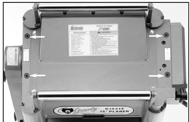
**Figure 41.** Feed roller lubrication points.
