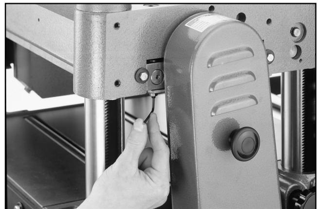
**Figure 24.** Feed roller height adjustment.
