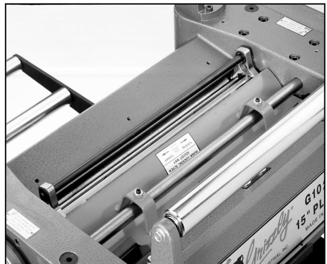
**Figure 15.** Cover Removed, Jig on cutterhead
