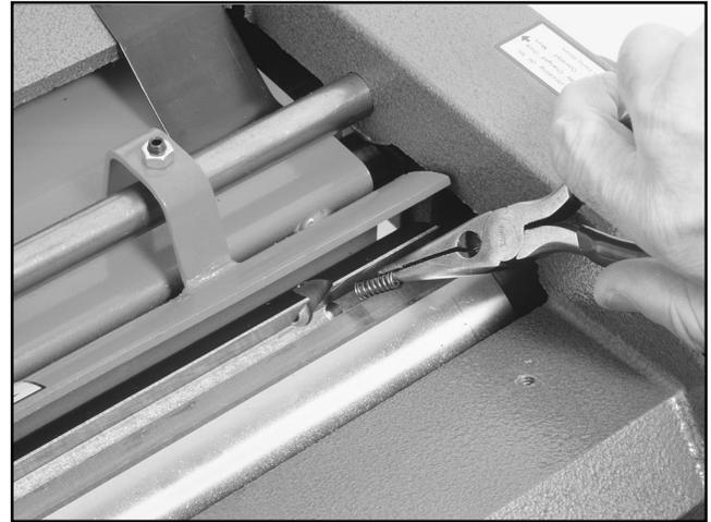
**Figure 14.** Placing springs into knife slots.
