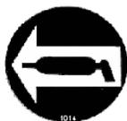
This symbol indicates a point that needs to be greased at an interval noted in the section below. Refer to the Detailed Maintenance section for further instructions on greasing. Copy and use the Daily Maintenance sheet located at the end of this section.
