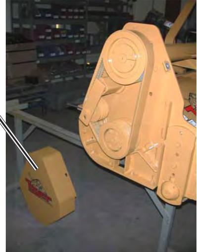
Place a straight edge over both sheaves and measure the belt tension (See TENSIONER MEASUREMENT PROCEDURE). To adjust the Rosta Tensioner, first, loosen the Rosta Stop and Rosta bolt that secures the Rosta to the flail. Next use the Wrench (PN# 06401023 available) to adjust the tension of the belt. After the tension has been set, secure the Rosta Stop and re-torque the Rosta Bolt to specs.
