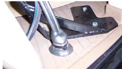
Next, wrap the cables with the 6" split hose at the point they pass through the hole, and secure the zip-ties. Apply RTV sealer in and around individual cables and split hose, inside and outside of the cab for a water tight seal. Install upper support bracket from cab post to the control lever stand.
